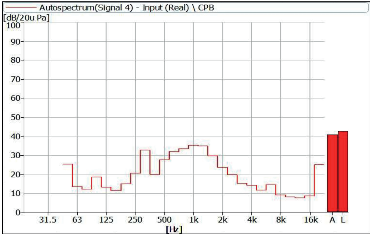
Figure 13 Noise Spectrum of Stage Luminaires (The Stage mode, Static, No 3)
