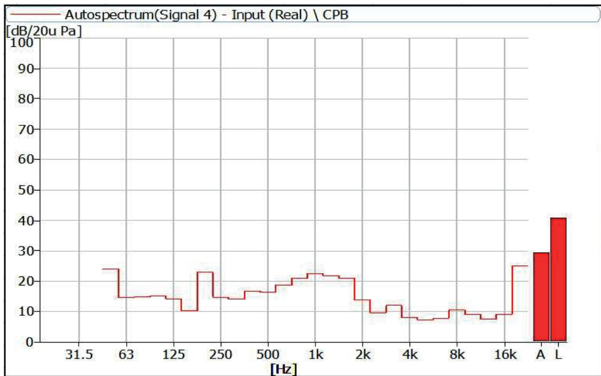
Figure 22 Noise Spectrum of Stage Luminaires (The Silence mode, Static, No 4)
