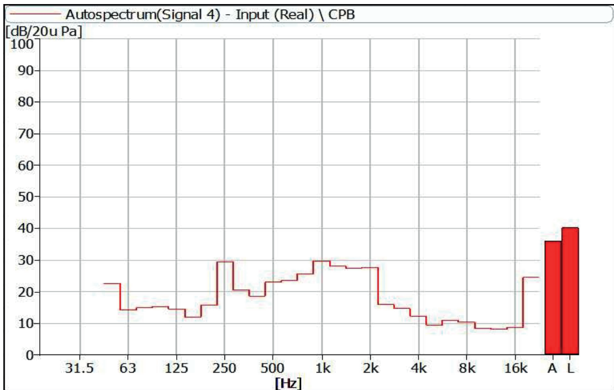
Figure 6 Noise Spectrum of Stage Luminaires (The Auto mode, Static, No 4)
