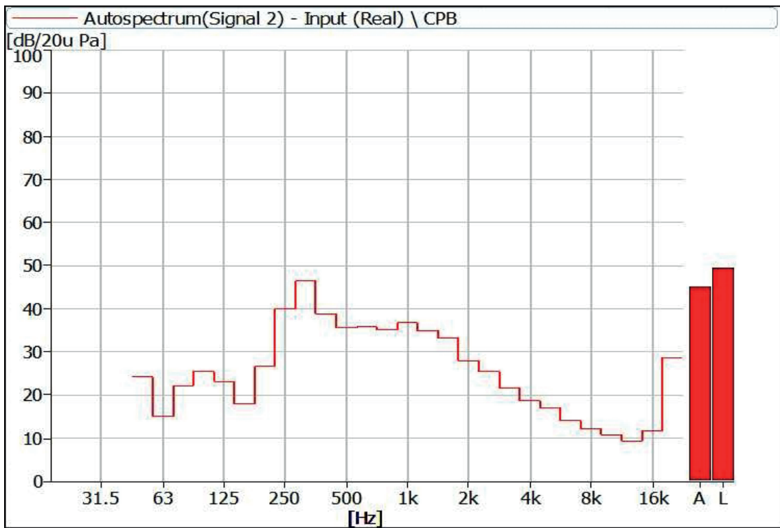
Figure 16 Noise Spectrum of Stage Luminaires (The Stage mode, Dynamic, No 2)
