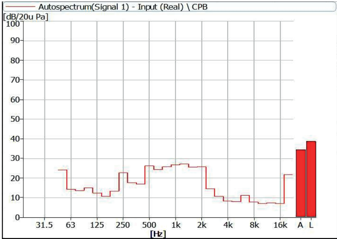
Figure 3 Noise Spectrum of Stage Luminaires (The Auto mode, Static, No 1)
